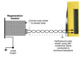
Figure 11 - Regeneration resistor connections
